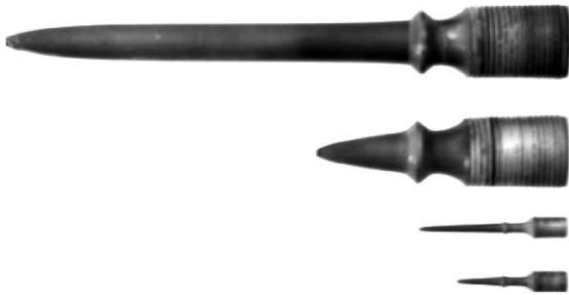
Fig. 12. Specimens type C1009, and C2024, \sigma = 25 MPa, 700 °C.
