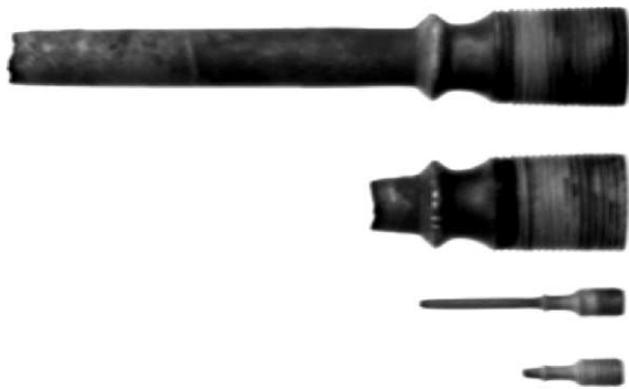
Fig. 13. Specimens type C1033, and C2030, \sigma = 15 MPa, 800 °C.
