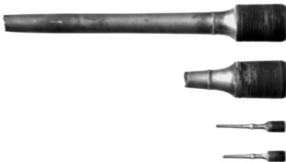
Fig. 14. Specimens type C1001, and C2001, \sigma = 25 MPa, 900 °C.
